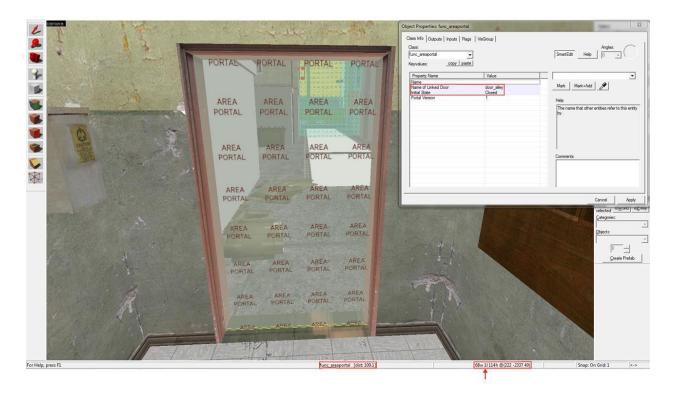
If you check the red arrow on the screenshot, it shows you that the areaportal thickness is 1 unit, which is perfect to completely hide it inside the door. In the properties window, you simply input the name of the door in the "name of linked door" field and you set the initial state to "closed". Please note that if your door starts open in the map, set the initial state to "open"; the areaportal state simply has to match the door's initial state.
