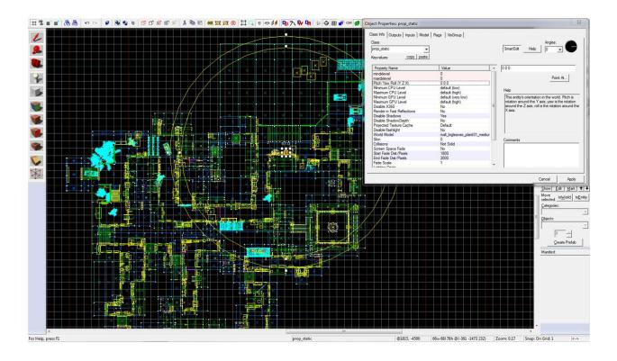
Since this is 2D, instead of spheres, you get here 2 flat circles showcasing the corresponding fade distances (again the radius of the circle is the fade distance). As a rule of thumb, always have the end fade distance to be higher than the start distance by at least 200 units; this will ensure a smooth transition while fading, otherwise, the fade effect will be abrupt and unrealistic in-game.
