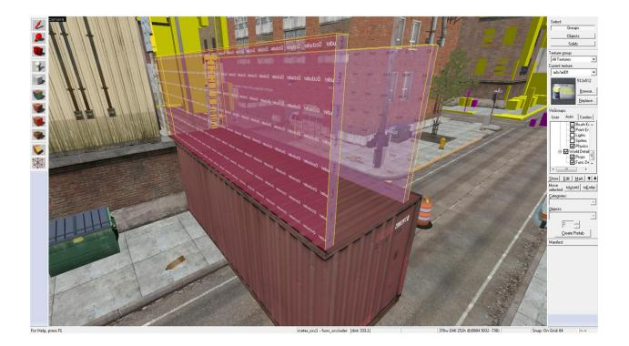
This shot is from cs\_assault. I temporarily removed the upper container so you can see the occluder that is inside (both containers include occluders). Please observe the texturing: the face on our side has the occluder texture while the other faces are "skipped". When you are standing near the dumpster, the occluding face will hide all props behind it within your viewing angle (default  $90^{\circ}$  for CS and  $75^{\circ}$  for HL2).
