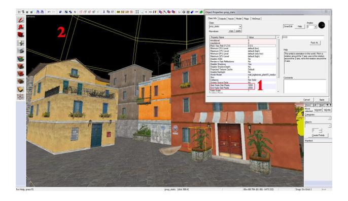
The highlighted rectangle labeled 1 is where you input the fade distance in Hammer units. These numbers mean that this prop will start fading at a distance of 1800 units from the player and will disappear completely at a distance of 2000 units; a prop that is not rendered will reduce engine overhead and increase fps.
