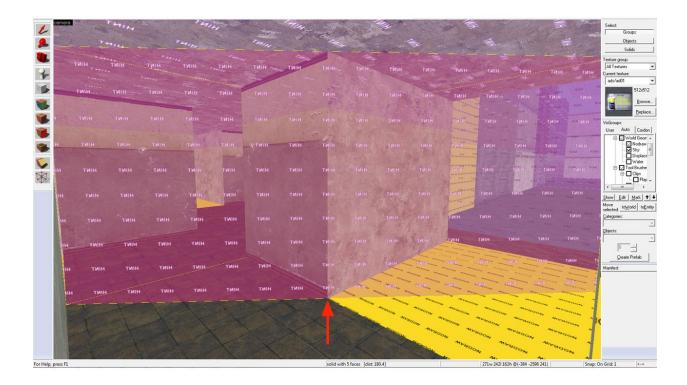
This is a typical indoor corner from de\_spezia\_pro. Notice how the face with hint texture is perfectly touching the tip of the corner (red arrow location); all the other faces of this triangle are textured with "skip" (unless you want another face to also cut visleaves, then you should texture it with hint).
