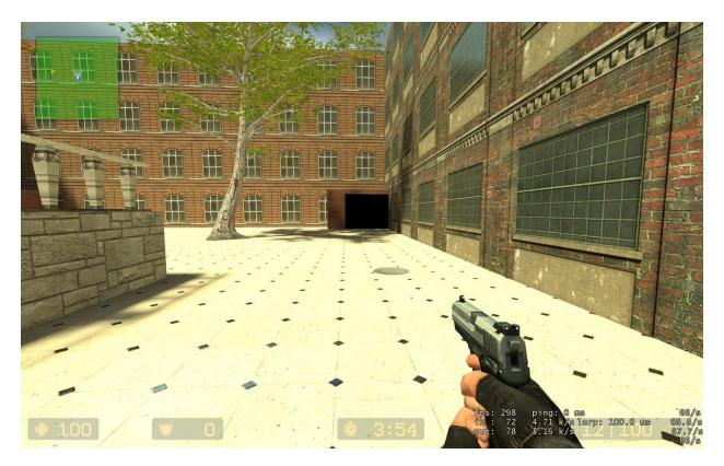
I am standing here beyond the end fade distance (1024 units in our example); the areaportal is fully closed and the black func\_brush is rendered instead.
