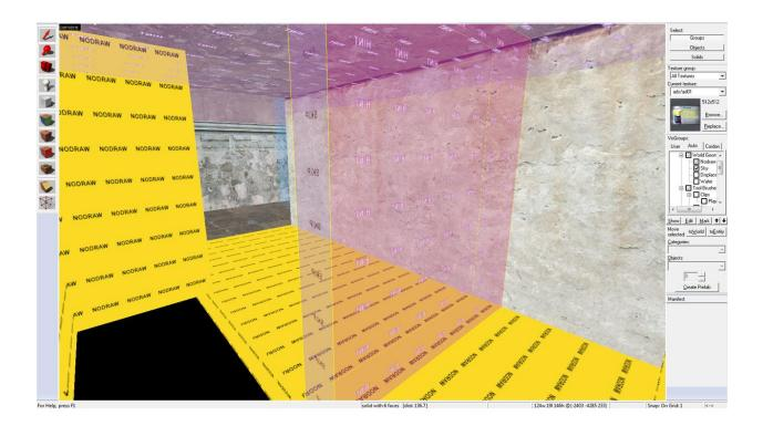
As you can see, it's a regular world brush, not an entity. The surface that is facing us has the hint texture while the other faces have the skip texture. The engine will cut the visleaf and separate it into 2 only on the hint face; the other skip faces are...well, skipped <sup>(2)</sup> (the engine will simply delete these faces in-game).
