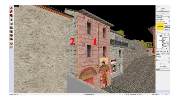
The brush labeled 2 is the world brush from the above screenshot acting as backbone to seal the level and as a support brush for the skybox and hints/areaportals. You can see that the thin brush labeled 1 is actually several func\_detail brushes to make it easier in manipulation and texture application.
