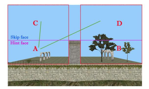
The only thing that changed is the addition of the horizontal hint brush that is neatly lying on the middle wall's top (hint face down, skip face up). The engine (vbsp more specifically) has now additional information to divide the A & B visleaves; we now have 4 visleaves: A, B, C & D. You can immediately see that A has direct LOS with C and D but not with B anymore (if you have to cross the skybox or world geometry, then it is not direct LOS anymore).
