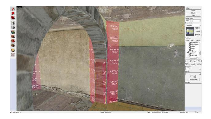
Arches also should be set to non-solid. 3 clip brushes will be placed to smooth the player's movement: 1 square in the middle to simulate the lower arch portion and 2 triangular on each side to allow players to slide on the angular face without getting stopped.
