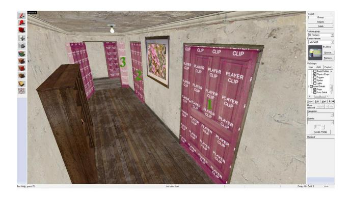
As we have seen in the door screenshot earlier, all doors that don't open should be clipped with a square brush that fits nicely inside the door's cavity. The doors labeled 1 and 2 are neatly clipped, the corner labeled 3 is also clipped with a triangular brush and the picture frame in between the doors is non-solid; the player will simply glide like a breeze through this corridor without anything tiny on the wall or floor stopping him.
