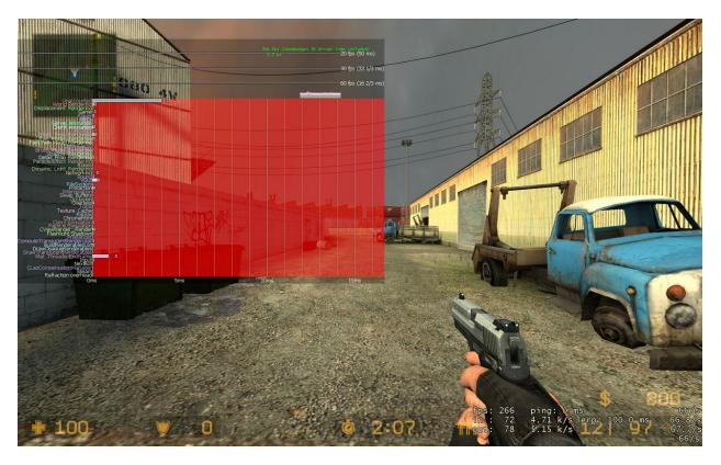
You can notice a decrease in overall fps of around 30 frames per second because, without occluders, the engine will render all the props that were hidden in the previous pic, since they are in visleaves that are seen by your visleaf. In this case, you can safely deduce that the occluder was needed here and was giving you a boost of 30 fps, totally justifying its cost.
