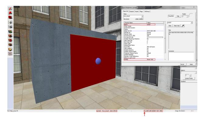
If we hide the areaportal in Hammer, we can finally see the linked brush. It must have a name, to be used to link it to the areaportal. The width is 3 units (red arrow location), just perfect to be completely enveloped inside the areaportal (8 units). The solidity should be set to "never solid" otherwise players won't be able to cross it, and the brush should be textured in black or white/grey-ish.
