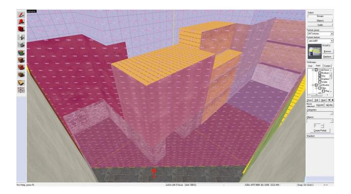
You can see in the above screenshot the triangular hint brush with the hint surface facing towards us while the other faces are "skipped". The red arrow points to the corner tip where the hint touches the corner edge. This setup will ensure that visleaves on both sides of this corner won't see each other. The player that is on one side won't have any content rendered from the other side, and this can only mean one thing: higher fps.
